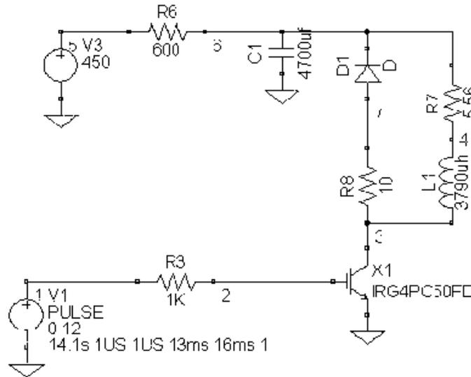
Figure 5. The solenoid controlling circuit design
