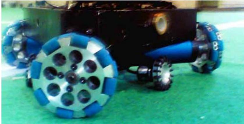
Figure 2 Three omni directional wheels act as actuators while three free wheels are for feedback.
