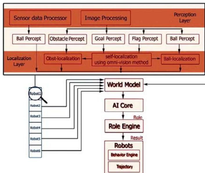
Figure 7. World model construction and artificial intelligent structure.
