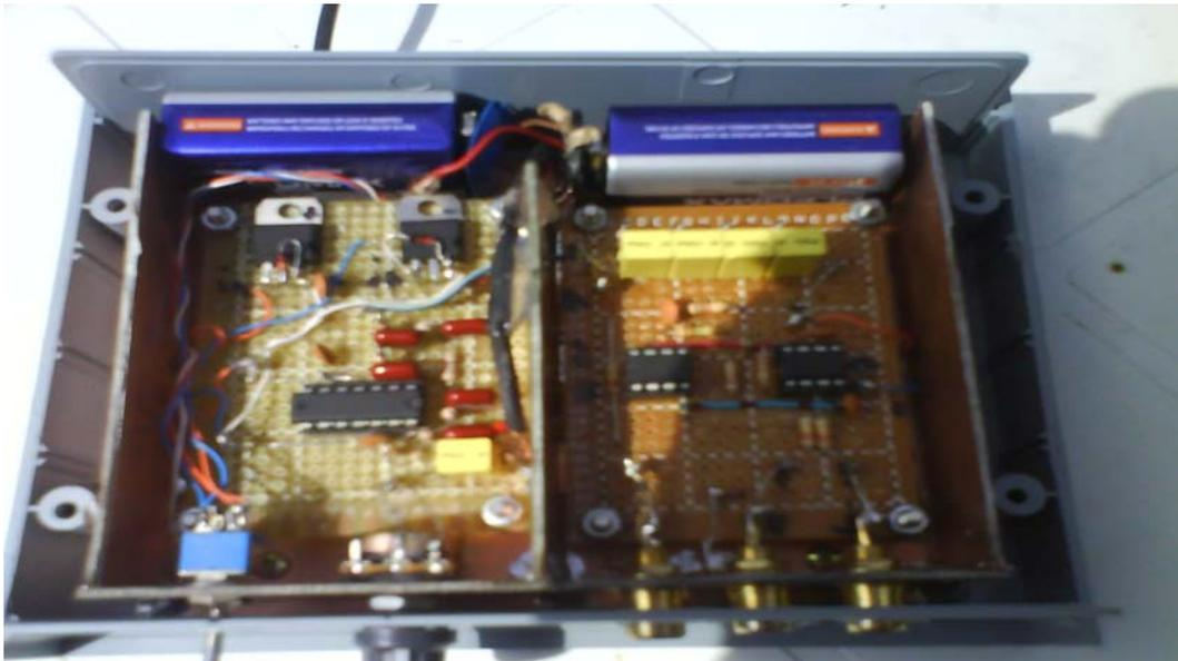
Figure 11. Practical realization of the EKG amplifier
