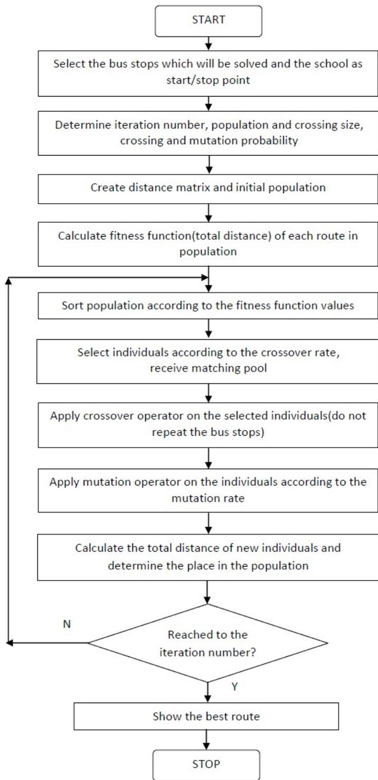
Figure 3. The flow diagram of the SBRP solution by using GA
