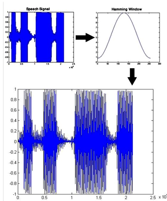
Figure 4. Hamming Window applied to each frame
