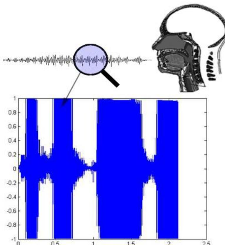
Figure 3 Frame blocking of the speech signal
