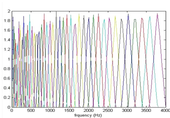
Figure 5. Mel-spaced filter bank
