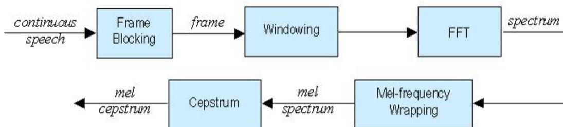
Figure 2. MFCC Block Diagram
