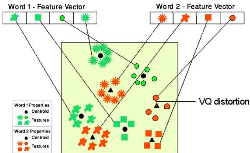
Figure 10. Conceptual diagram illustrating vector quantization codeword formation.
