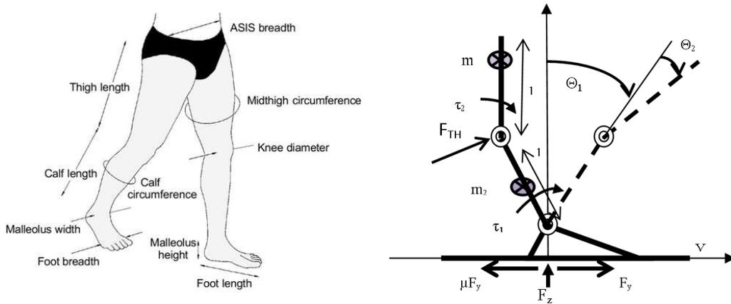
Figure 3: Anthropometric data of the lower extremity required for the prediction of body segment parameters and the model of human leg in walking process
