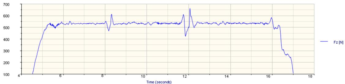
Figure 8: Variation of the contact force between the foot and support (subject with locomotion disability)
