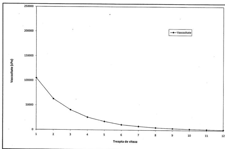
Figure 3: Viscosity variation depending on speed rate
