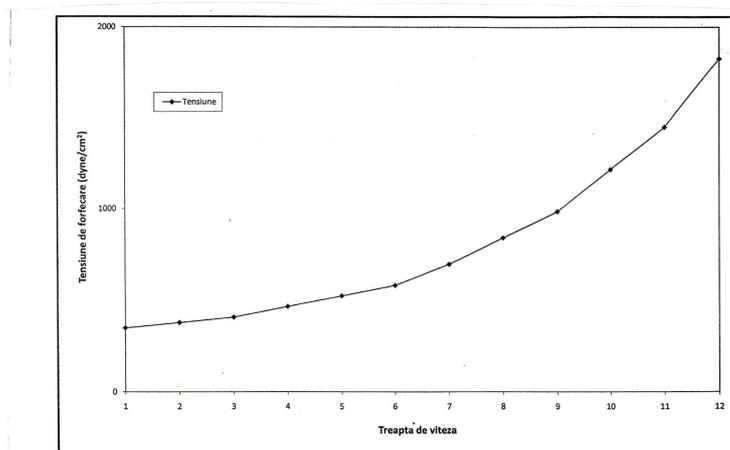
Figure 2: Variation of the shear stress depending on the speed rate
